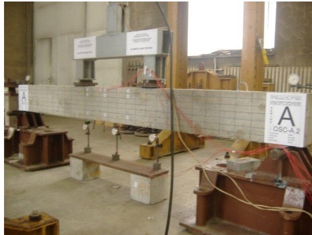
Slika 2. Prikaz grede prije ispitivanja s mjernim uređajima i nanošenje opterećenja Figure 2. Beam prior to the test with measuring devices and loading application
